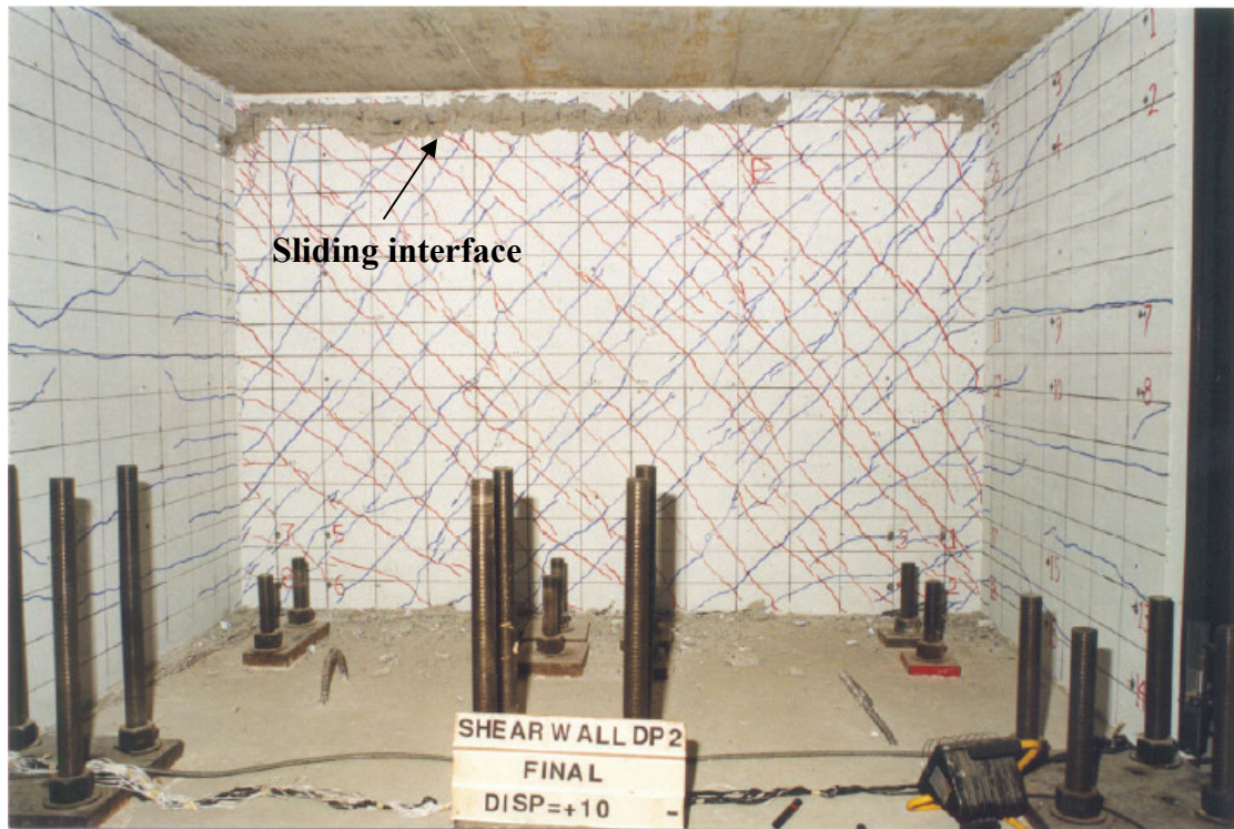
Figure 8 Cracking pattern for wall DP2 tested by Palermo and Vecchio (2002) at a sliding failure between the wall web and top slab
